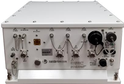
This Narda-MITEQ series of outdoor, antenna-mounted block upconverter is designed to cover simultaneously multiple wide bandwidth satellite transponders by accepting four independent IF inputs which are up converted into one wideband RF output.
